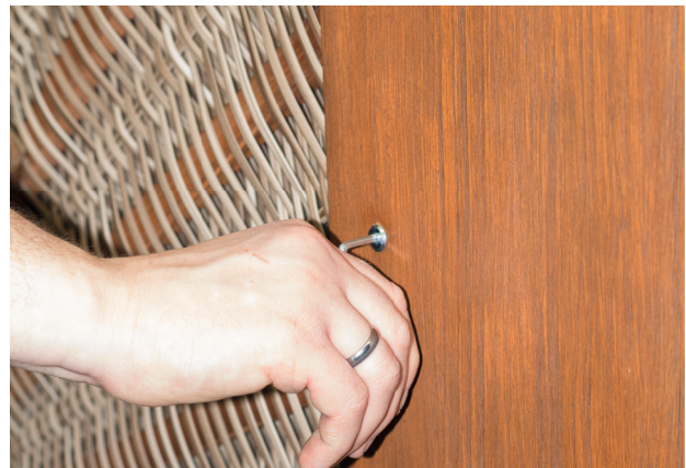
Loosen the side panels Step 3: Carefully unscrew all the remaining screws on the side panel
