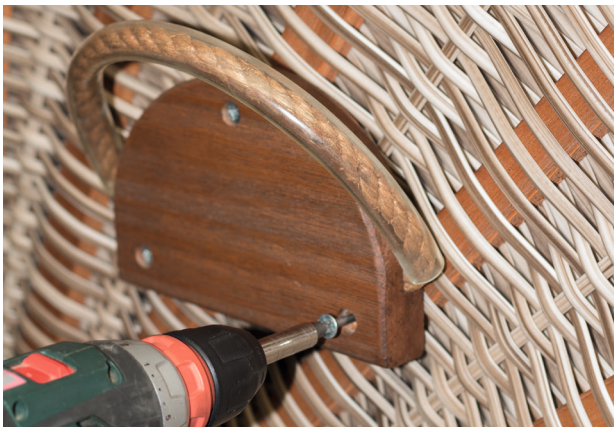
Loosen the side panels Step 2: Carefully unscrew the carrying handle
