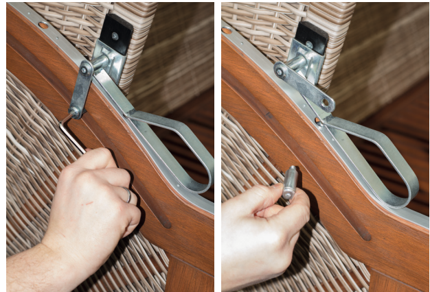
Loosen the side panels Step 1: Carefully unscrew the adjustment handle
